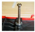
To test the nut for correct orientation, turn in a 3/4" or longer 2/56 screw. Use it as a "joystick" to tilt the nut so that the screw is in a true vertical position when observed from every angle. Once you've got it right, very gently turn out the screw, so as to avoid tilting the nut as you do so.
